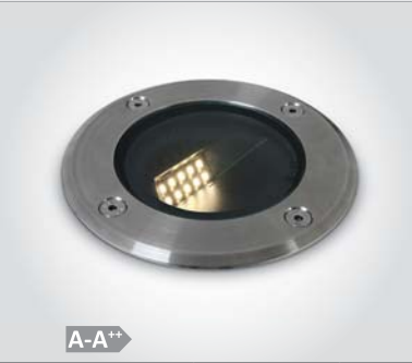
69062 | 8W | SMD 2835 | Assymetrical | Stainless steel 316 + Die cast
